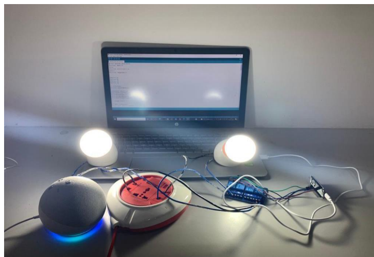
Fig6. Hardware Integration and controlling both lights using Alexa
